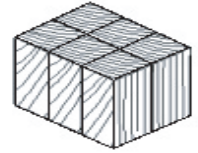
End Grain Sealed and Oiled (Minimum 3" Thick - Blocks 1 3/4" Square)
